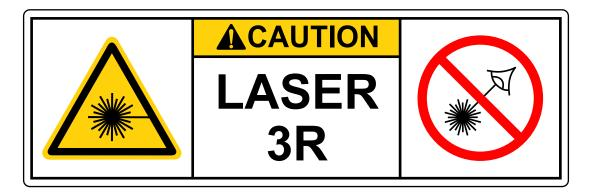
This product is intended for LASER shows only. The class 3R laser light should only be operated by professional operators.
